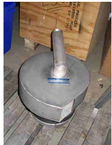
VHV with air vent for minimal slopes
