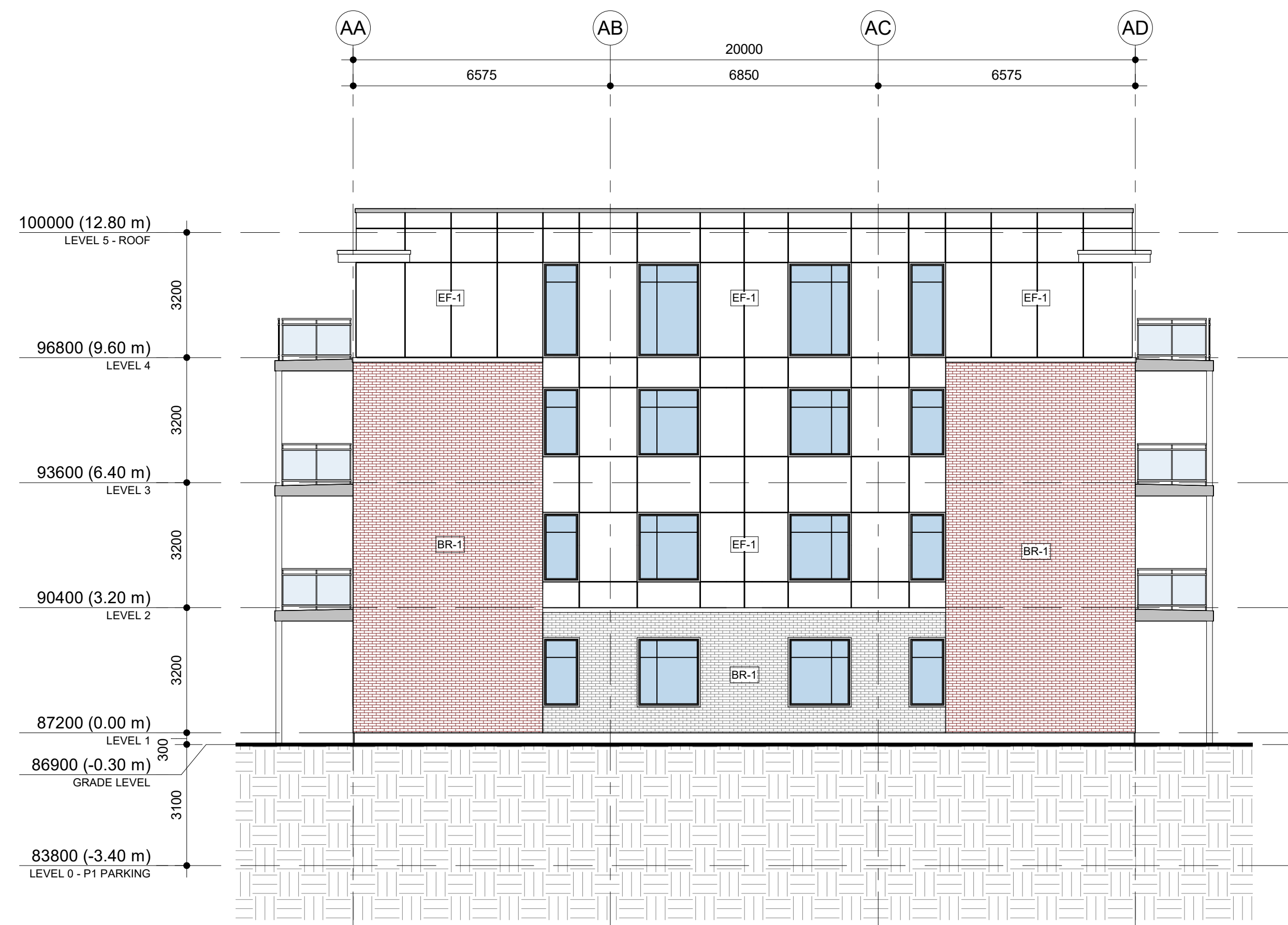
2 BUILDING A - SOUTH ELEVATION A201 1 : 100
