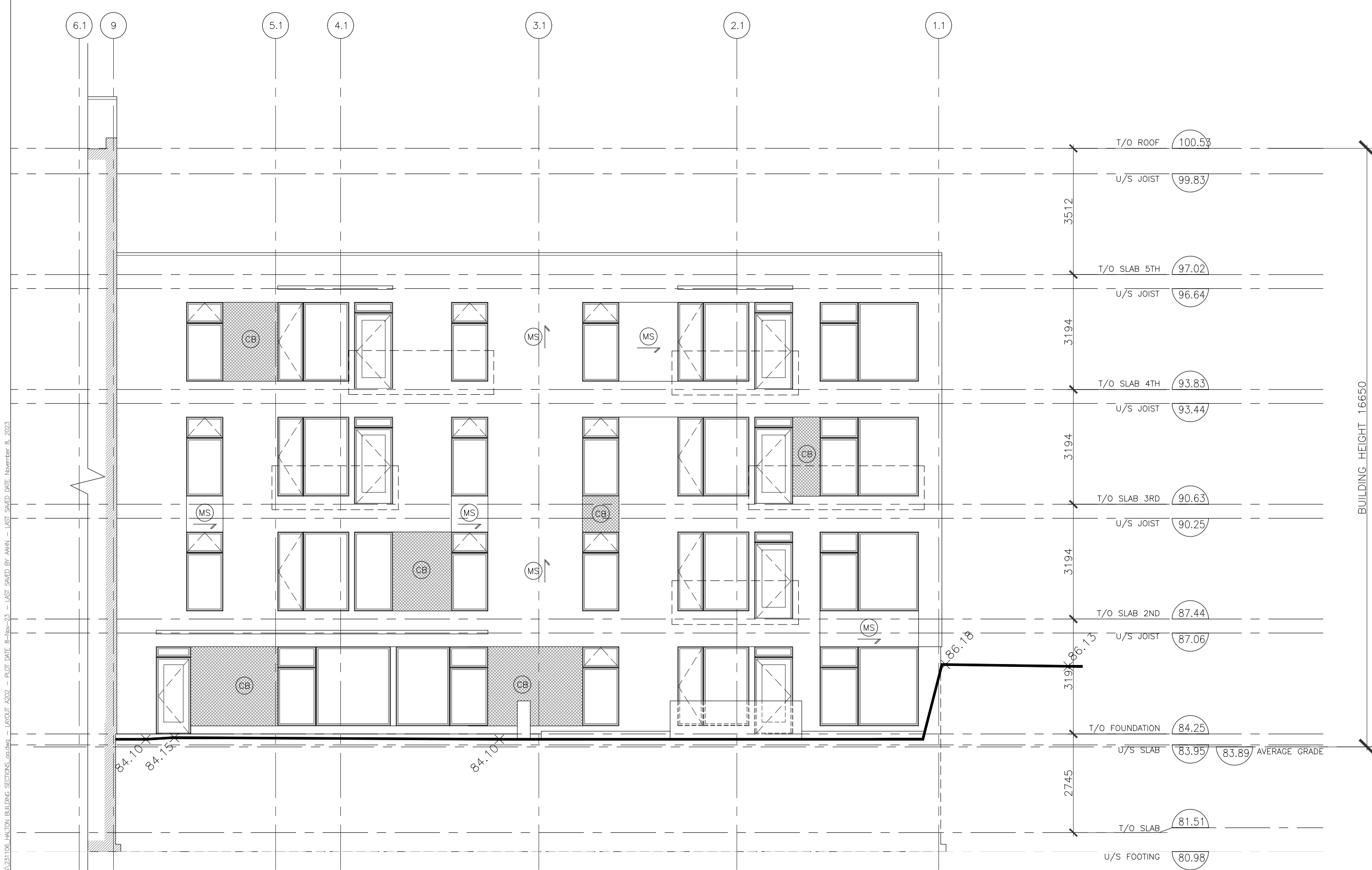
2 EAST COURTYARD ELEVATION 1:100
