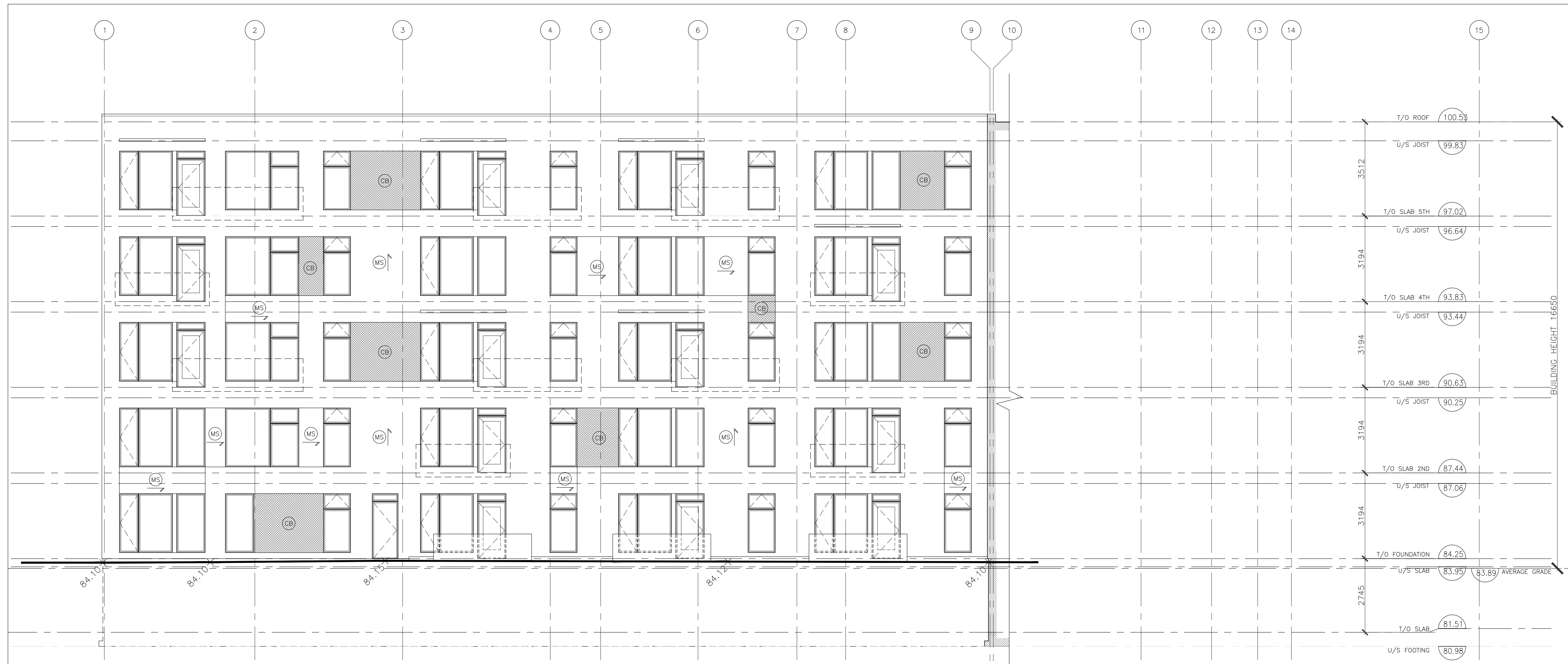
1 WEST COURTYARD ELEVATION 1:100
