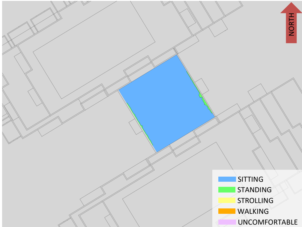
FIGURE 5A: SPRING – WIND COMFORT, LEVEL 2 AMENITY TERRACE
