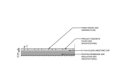
5 PROPOSED PRECAST CONCRETE PAVERS ON CONCRETE SLAB
