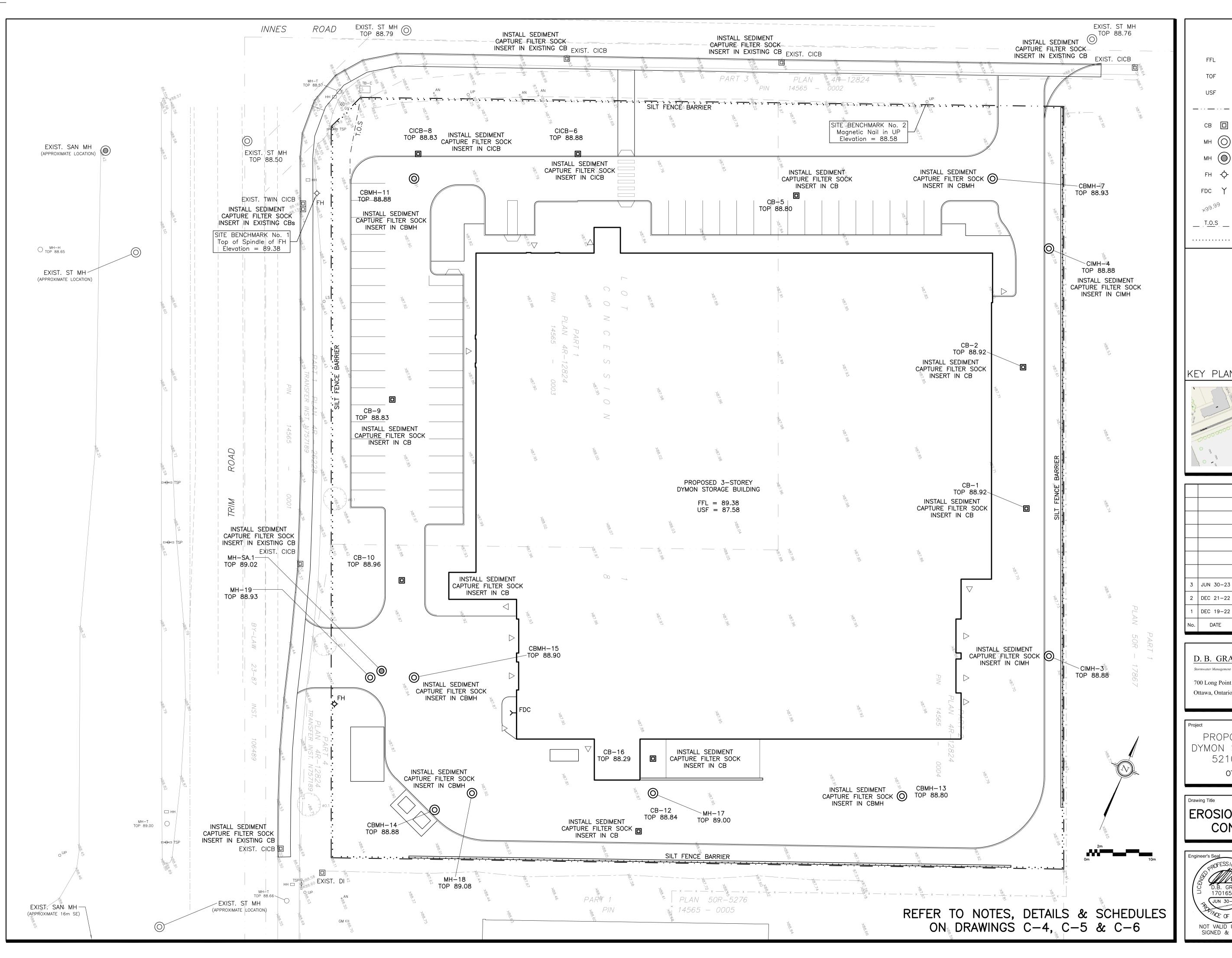
**LEGEND** FINISHED FLOOR ELEVATION TOP OF FOUNDATION UNDERSIDE OF FOOTING - · · - PROPERTY LINE CB CATCH-BASIN STORM MANHOLE ( ) SANITARY MANHOLE FH -O- FIRE HYDRANT FIRE DEPARTMENT CONNECTION EXISTING GRADE ELEVATION TOP OF SLOPE ····· SILT FENCE BARRIER KEY PLAN
