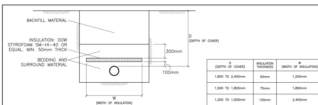
INSULATE WATERMAINS AND WATER SERVICES AS INDICATED AND WHERE DEPTH OF COVER IS LESS THAN 2,400mm.
