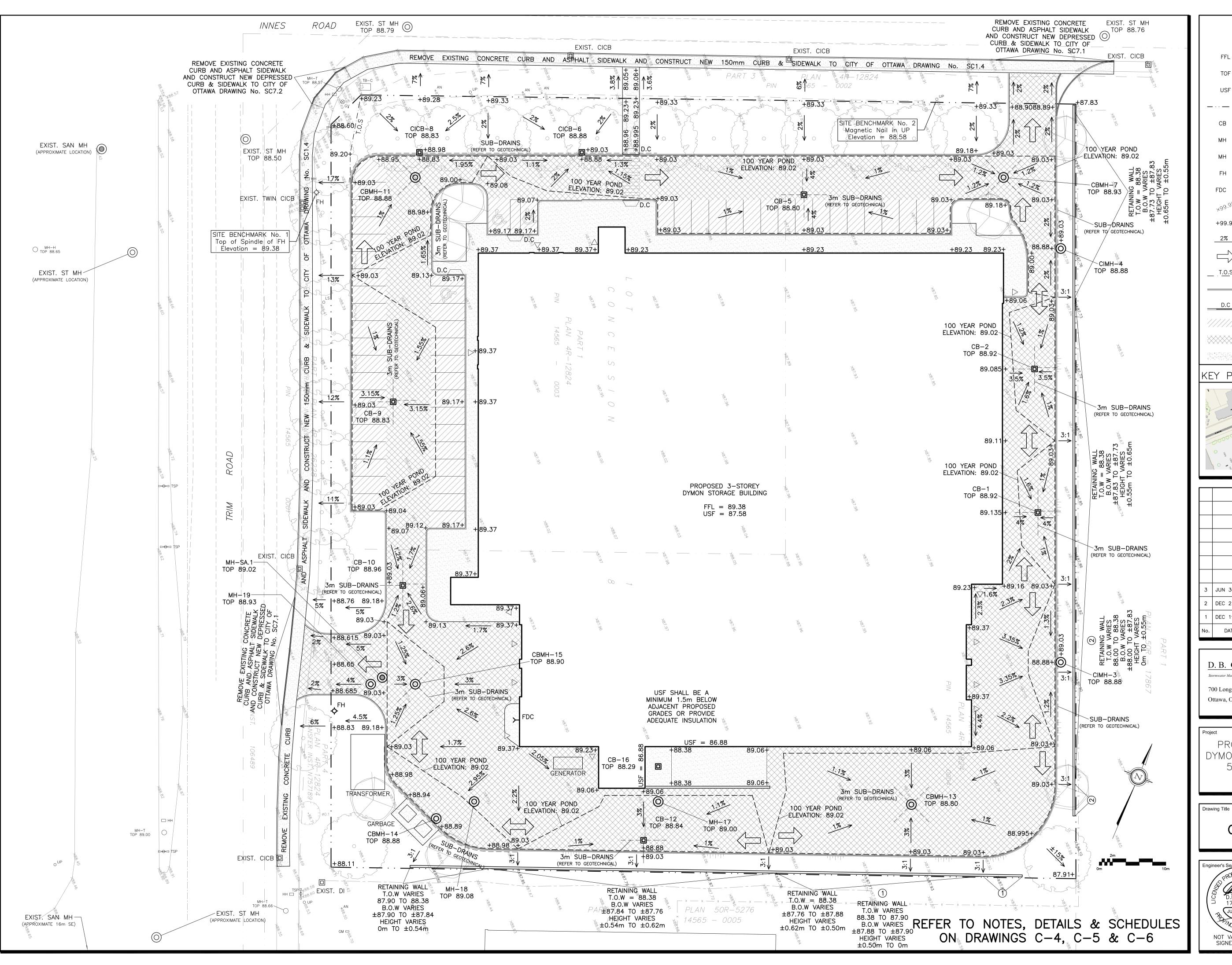
**LEGEND** FINISHED FLOOR ELEVATION TOP OF FOUNDATION UNDERSIDE OF FOOTING - · · - PROPERTY LINE CATCH-BASIN STORM MANHOLE SANITARY MANHOLE FH -O- FIRE HYDRANT FDC Y FIRE DEPARTMENT CONNECTION EXISTING GRADE ELEVATION PROPOSED GRADE ELEVATION PROPOSED SLOPE OF GRADE EMERGENCY OVERLAND FLOW TOP OF SLOPE 150mm BARRIER CURB DEPRESSED CURB MEDIUM DUTY PAVEMENT HEAVY DUTY PAVEMENT CONCRETE KEY PLAN
