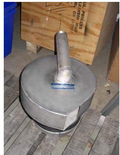
VHV with air vent for minimal slopes
