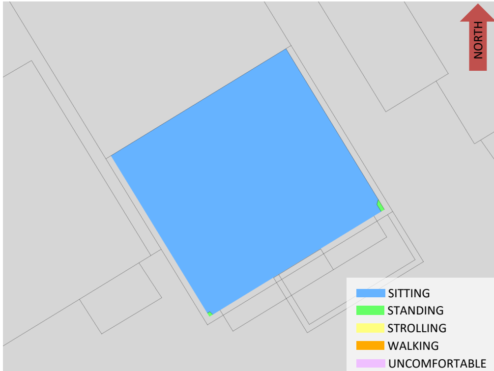
FIGURE 7C: AUTUMN – WIND COMFORT, MPH LEVEL AMENITY TERRACE
