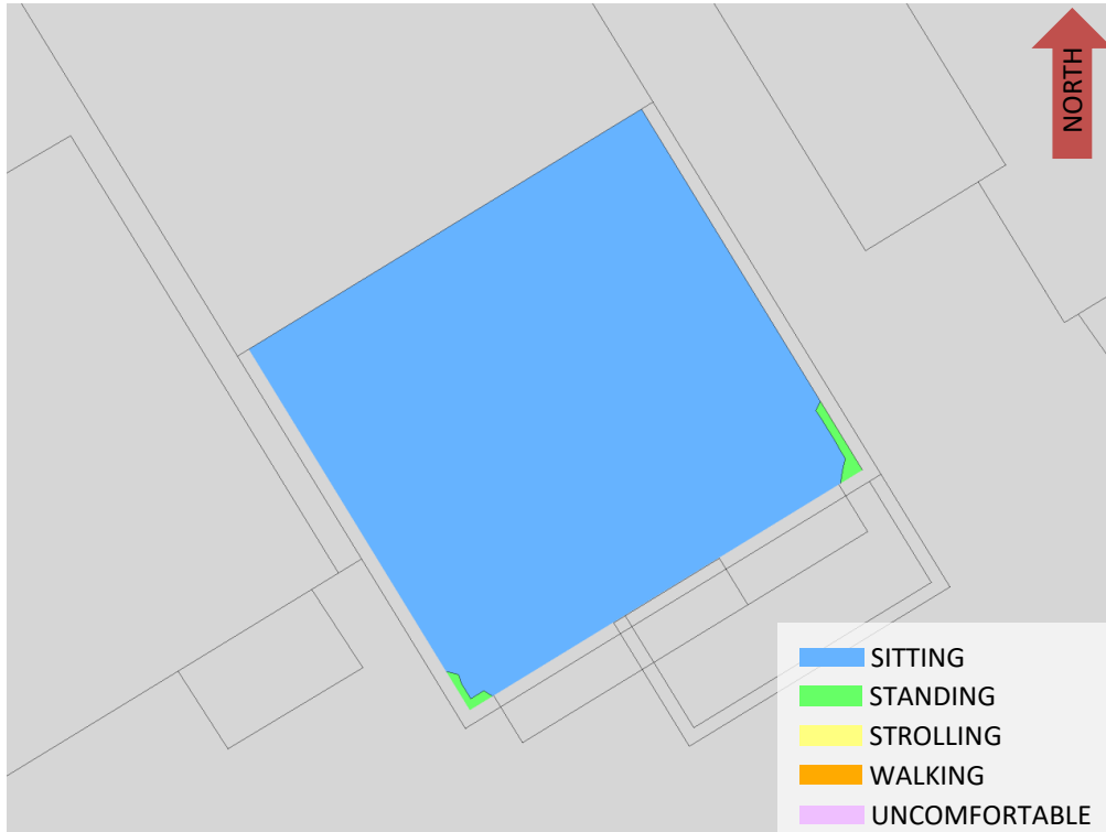
FIGURE 7A: SPRING – WIND COMFORT, MPH LEVEL AMENITY TERRACE
