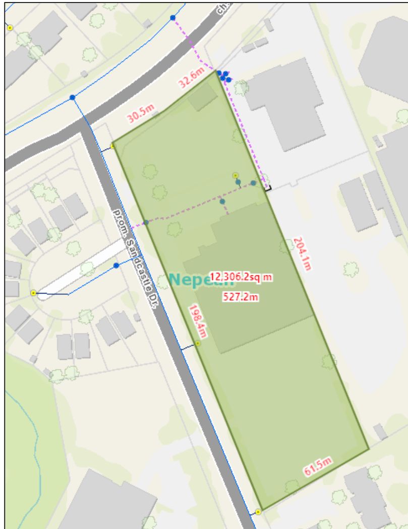
Figure 3-1: Fire Hydrant Coverage Sketch
