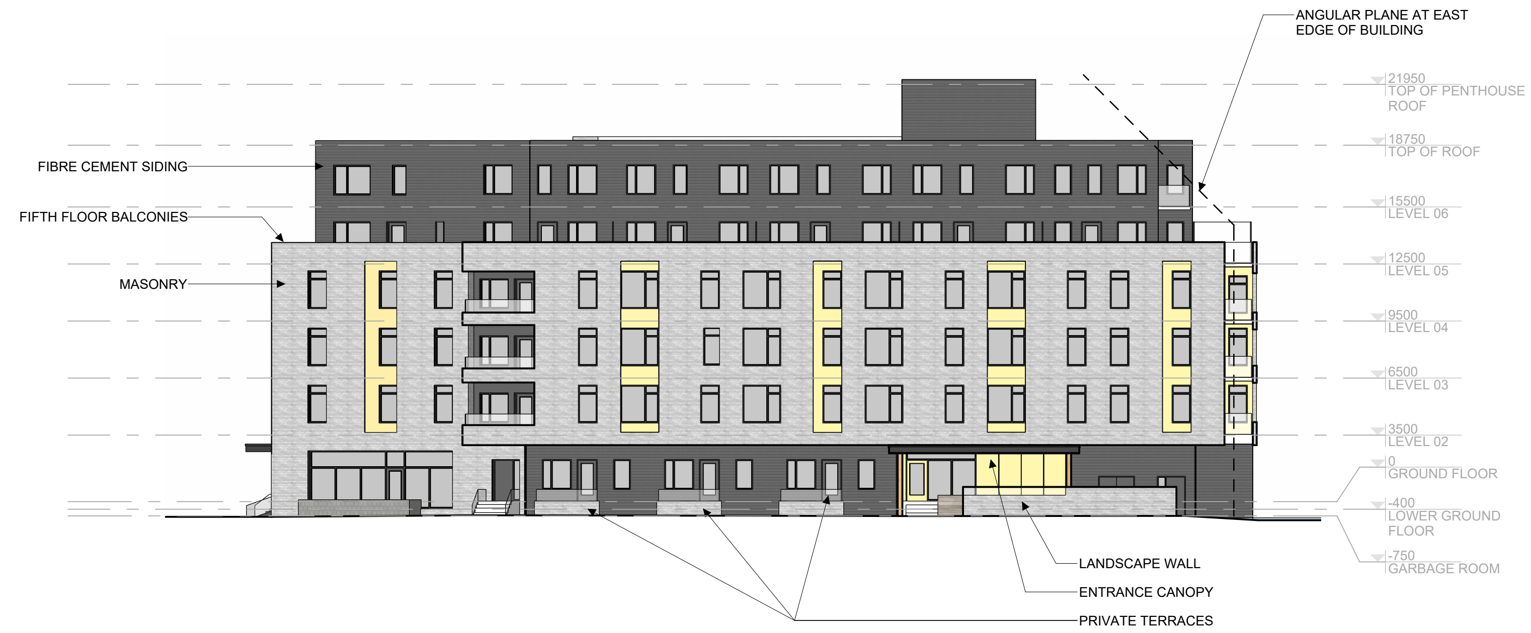
2 EAST ELEVATION A.300 | 1:200
