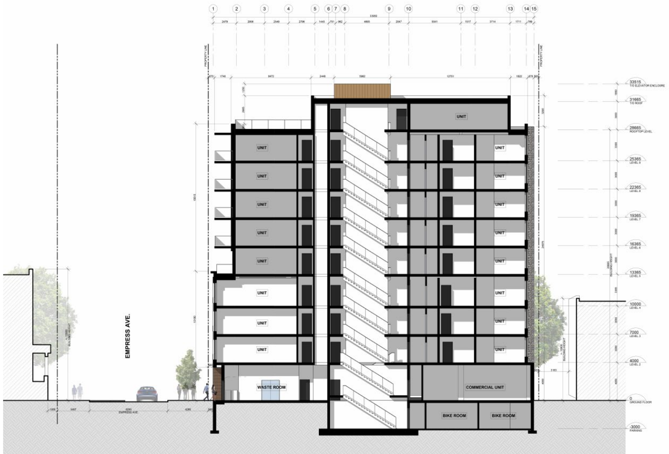
Figure 17: Building and Street Section – Empress Avenue
