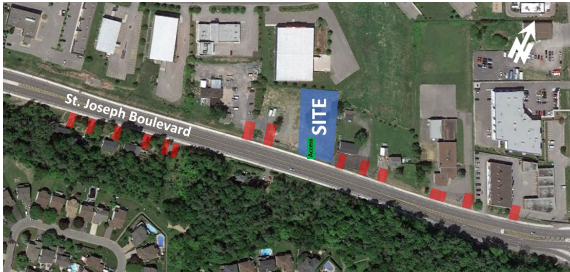
Figure 3: Adjacent Driveways within 200m of Site Access
