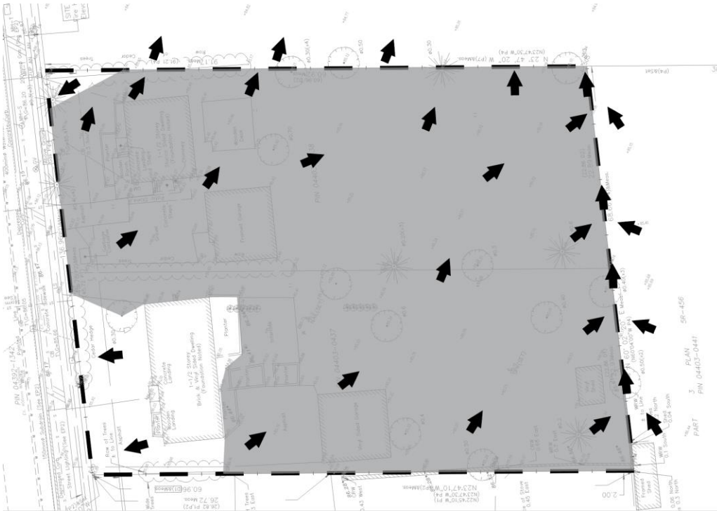
DRAINAGE TO NE PROPERTY IN EXSITING CONDITIONS (APPROXIMATELY 0.24ha)
