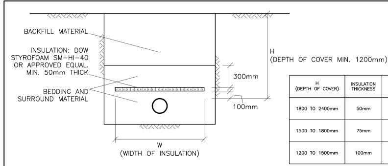
INSULATION (DEPTH OF COVER) (WIDTH OF INSULATION) 1800 TO 2400mm 1200mm 1500 TO 1800mm 1800mm 1200 TO 1500mm
