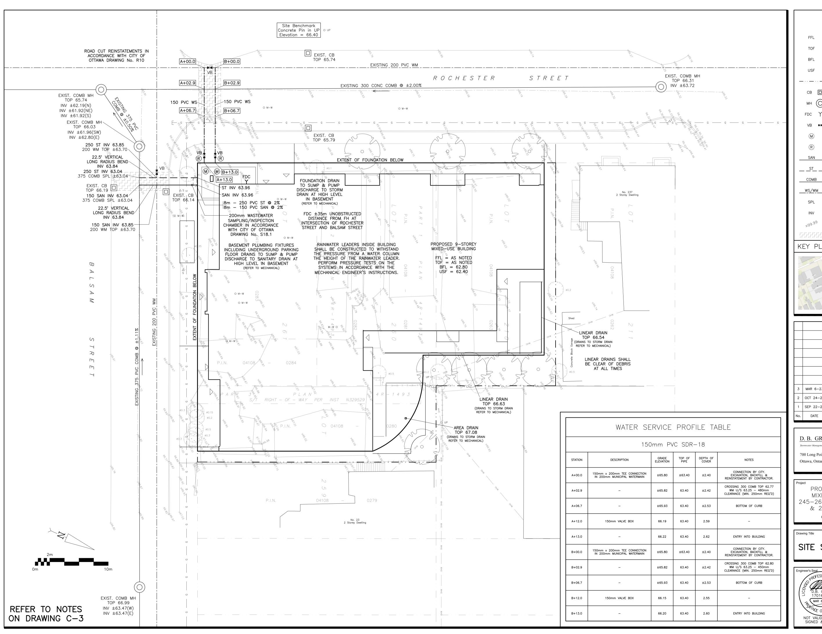
**LEGEND** FINISHED FLOOR ELEVATION TOP OF FOUNDATION BASEMENT FLOOR ELEVATION UNDERSIDE OF FOOTING CB CATCH-BASIN MANHOLE FIRE DEPARTMENT CONNECTION VB ■ VALVE & VALVE BOX WATER METER REMOTE WATER METER SANITARY SEWER SERVICE \_\_\_\_ST\_\_\_ STORM SEWER SERVICE COMBINED SEWER WS/WM WATER SERVICE/WATERMAIN SPRINGLINE OF PIPE INVERT OF PIPE EXISTING GRADE ELEVATION ROAD CUT REINSTATEMENT KEY PLAN
