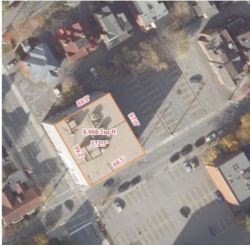
Figure 13: Existing Office Building Area Measurement
