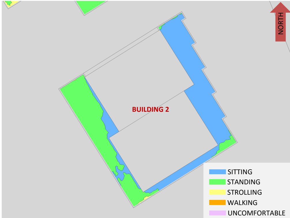
FIGURE 10C: AUTUMN – WIND COMFORT, BUILDING 2 LEVEL 5 AMENITY TERRACE
