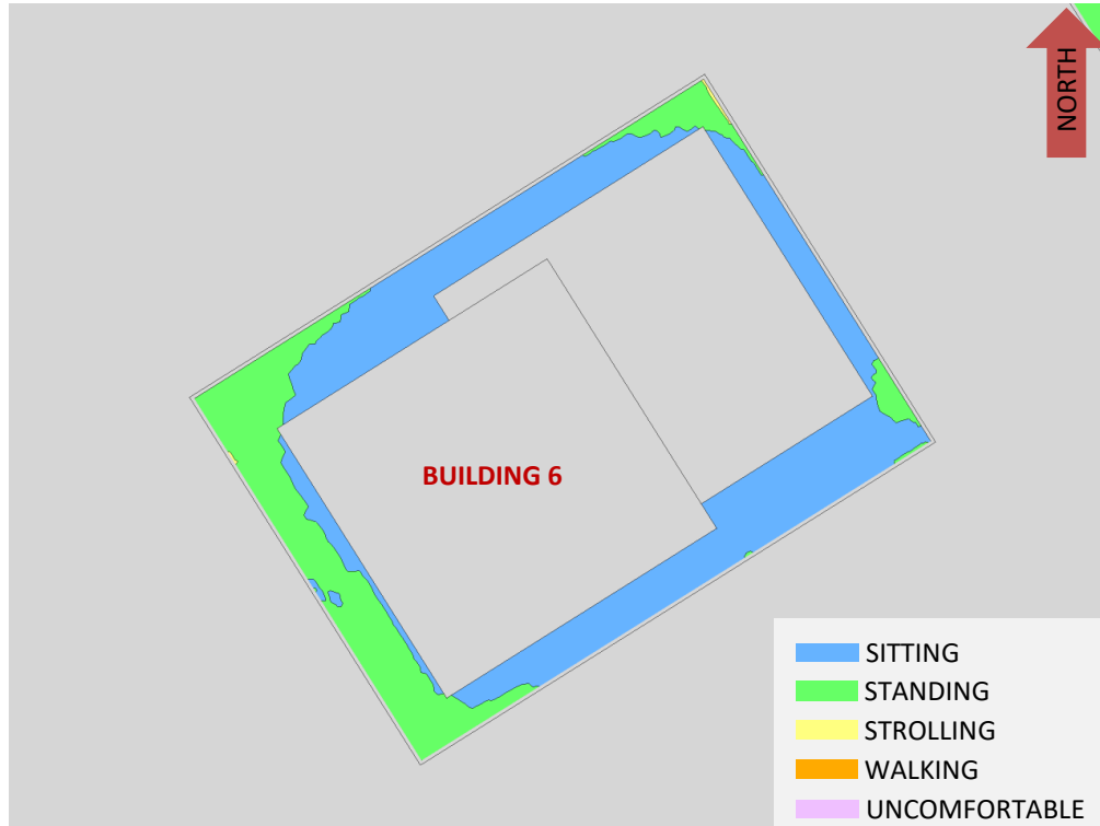
FIGURE 17: TYPICAL USE PERIOD – BUILDING 6 LEVEL 7 AMENITY TERRACE
