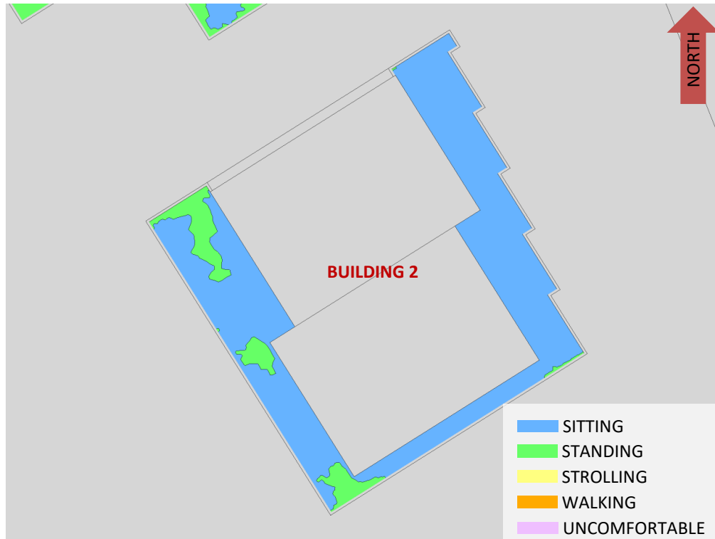
FIGURE 11: TYPICAL USE PERIOD – BUILDING 2 LEVEL 5 AMENITY TERRACE
