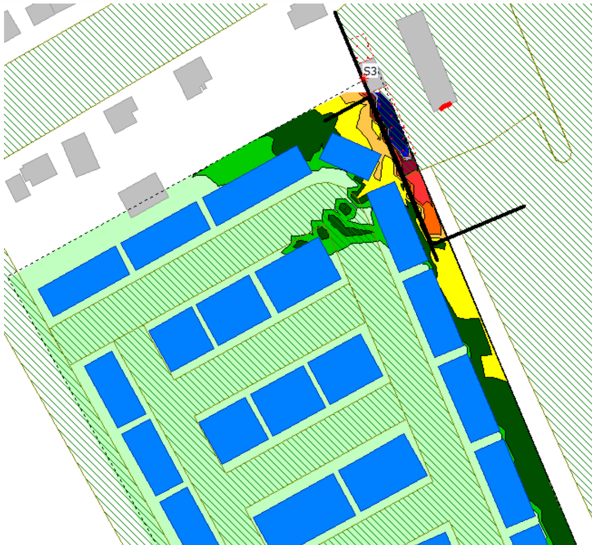
FIGURE 9: DAYTIME STATIONARY NOISE CONTOURS WITH PROPOSED 3M NOISE WALL (1.5 M ABOVE GRADE)
