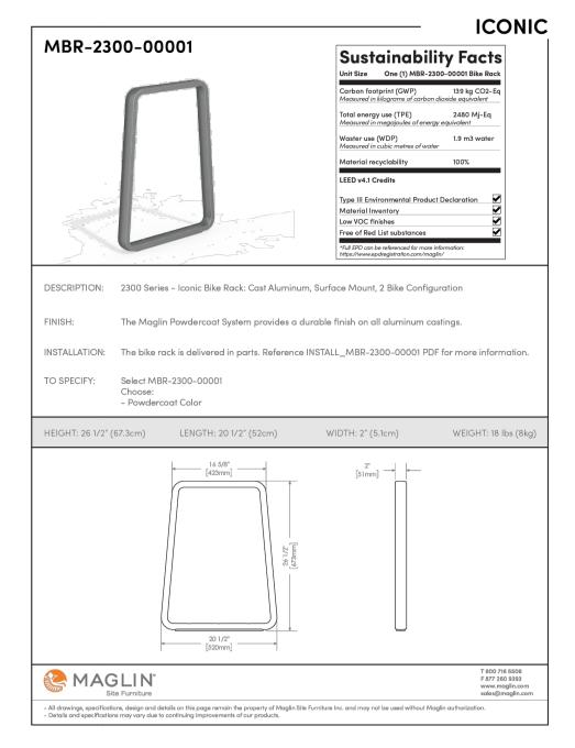
NOTES: SURFACE MOUNT TO CONCRETE PAVING WITH STAINLESS STEEL, TAMPER PROOF HARDWARE
