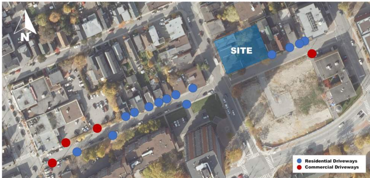
Figure 3: Existing Driveways to Adjacent Developments
