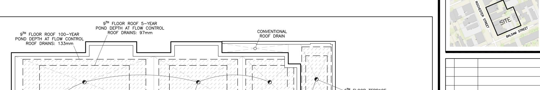
6<sup>TH</sup> FLOOR TERRACE FLOW CONTROL ROOF DRAINS WATTS RD-100 C/W ADJUSTABLE ACCUTROL WEIR CLOSED 0.31545L/s (5USgpm) PENTHOUSE ROOF 100-YEAR POND DEPTH AT FLOW CONTROL-6<sup>TH</sup> FLOOR ROOF 100-YEAR ROOF DRAINS: 137mm POND DEPTH AT FLOW CONTROL ROOF DRAINS: 139mm PENTHOUSE ROOF 5-YEAR POND DEPTH AT FLOW CONTROL-ROOF DRAINS: 101mm 6<sup>TH</sup> FLOOR ROOF 5-YEAR POND DEPTH AT FLOW CONTROL ROOF DRAINS: 101mm
