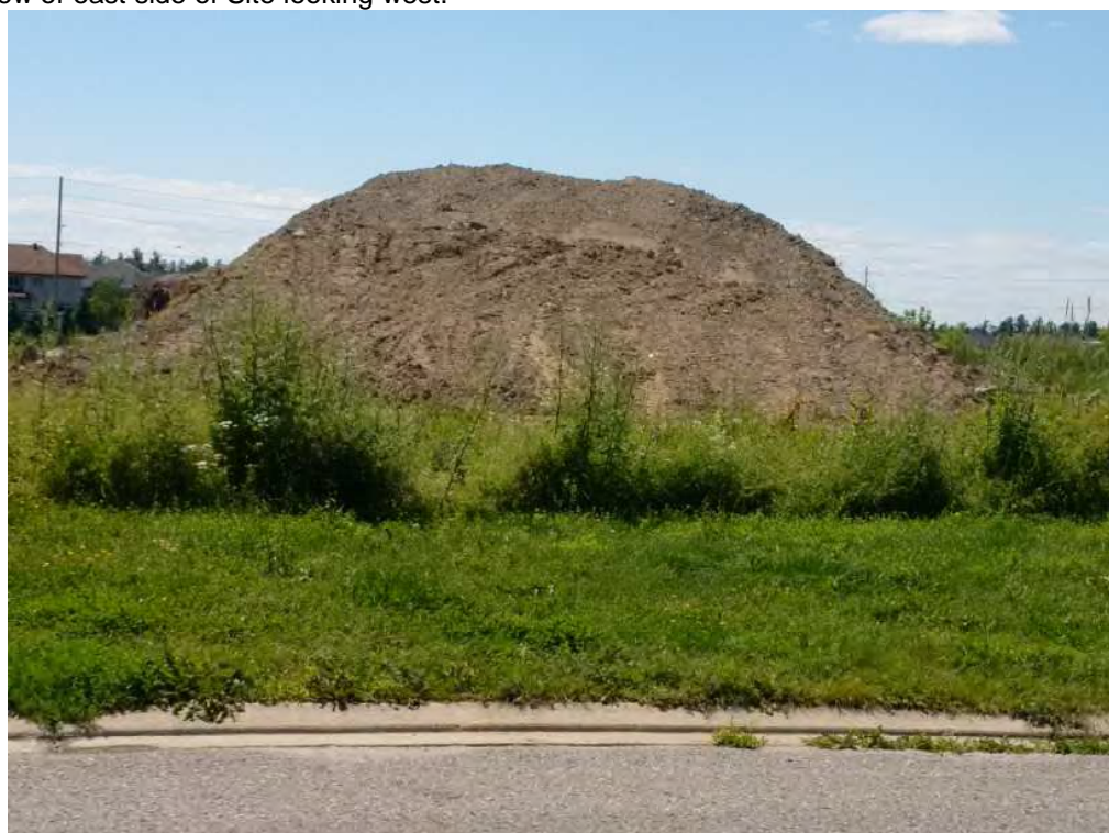
Photo 8: Off-site stockpile of sandy fill. No evidence of waste debris or contamination.
