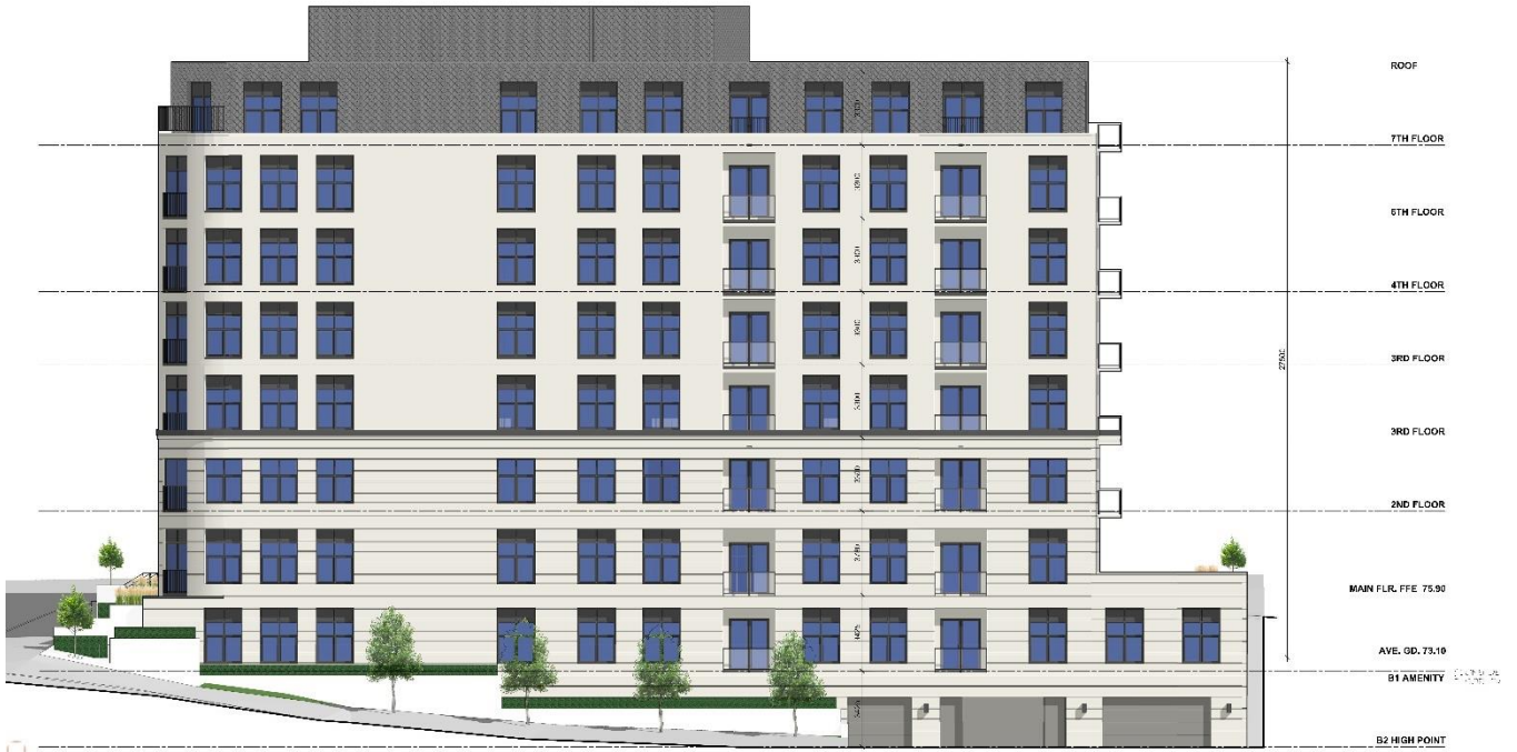
Figure 14: North elevation of proposed development
