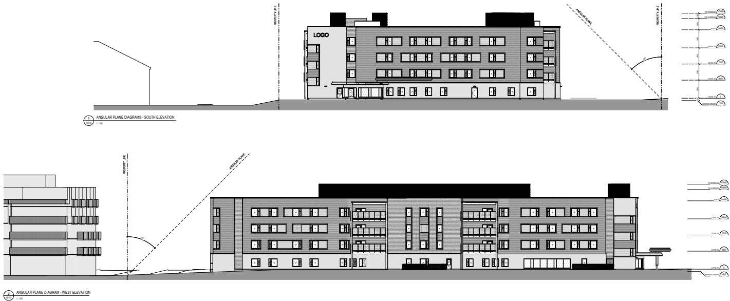
Figure 5.3 : Angular Plane Diagram, South and West Elevations illustrating how the proposed development provided for respectful transition to both existing and planned developments
