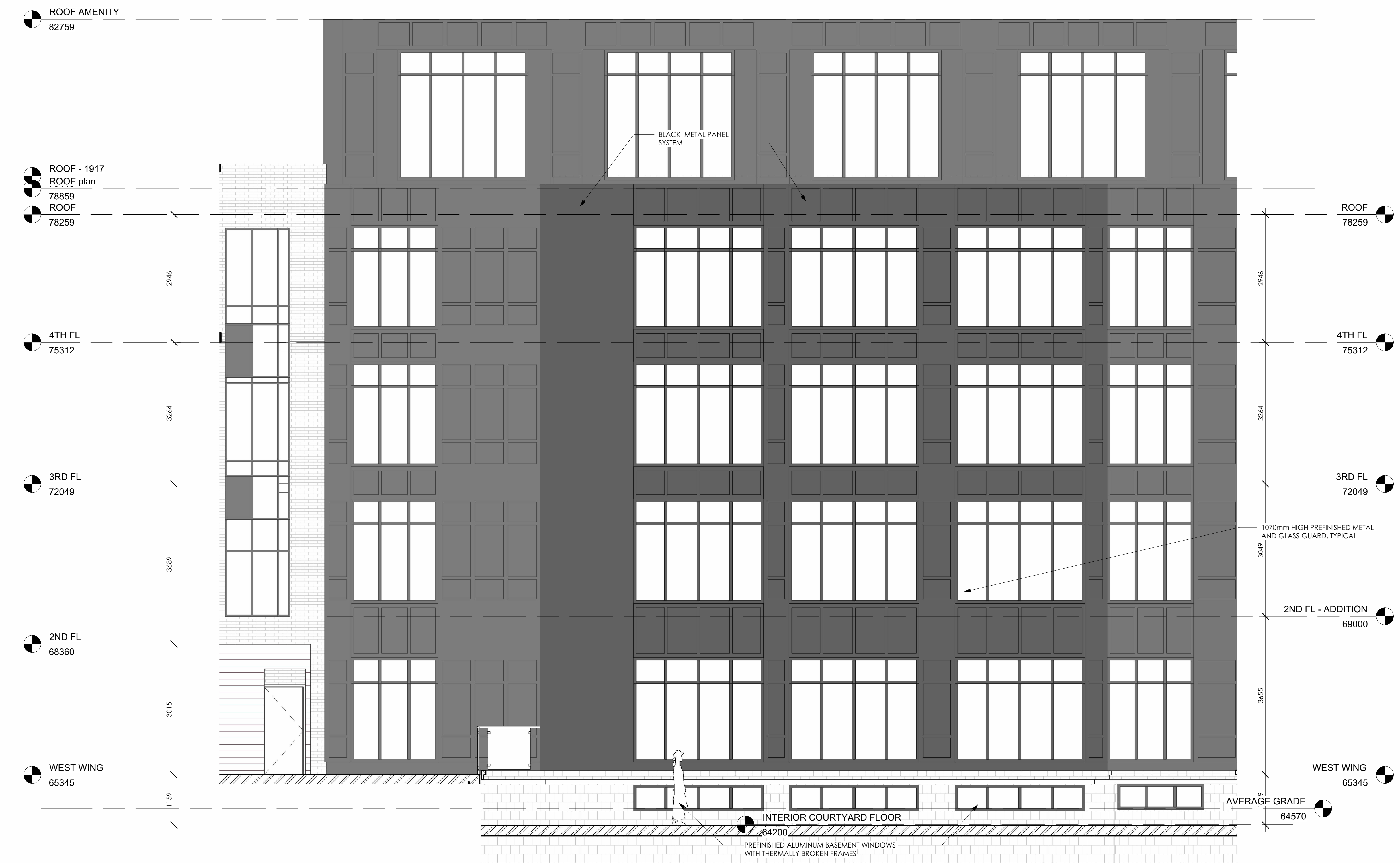
2 COURTYARD WEST ELEVATION 1 : 50
