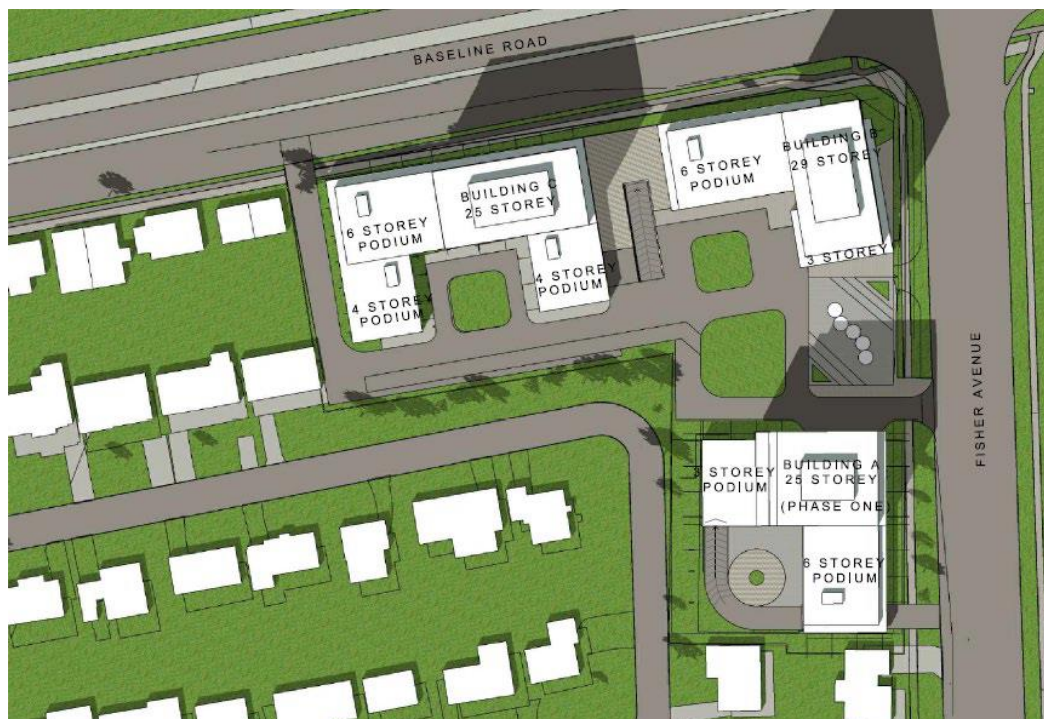
Figure 10: Site plan illustrating the full build-out of the property with two towers along Baseline and a 25-storey setback along Fisher Avenue. Source: Rodrick Lahey Architect Inc. 2022
