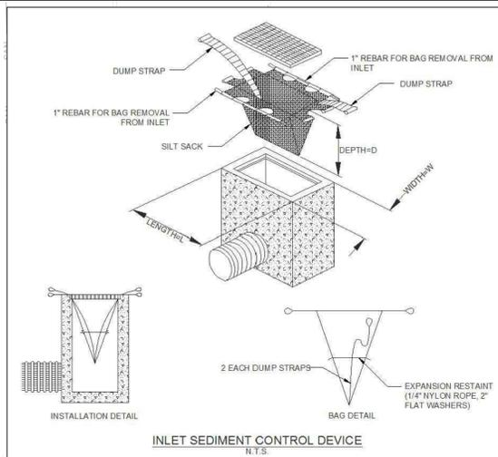
**EROSION AND SEDIMENT CONTROL MEASURES:**
