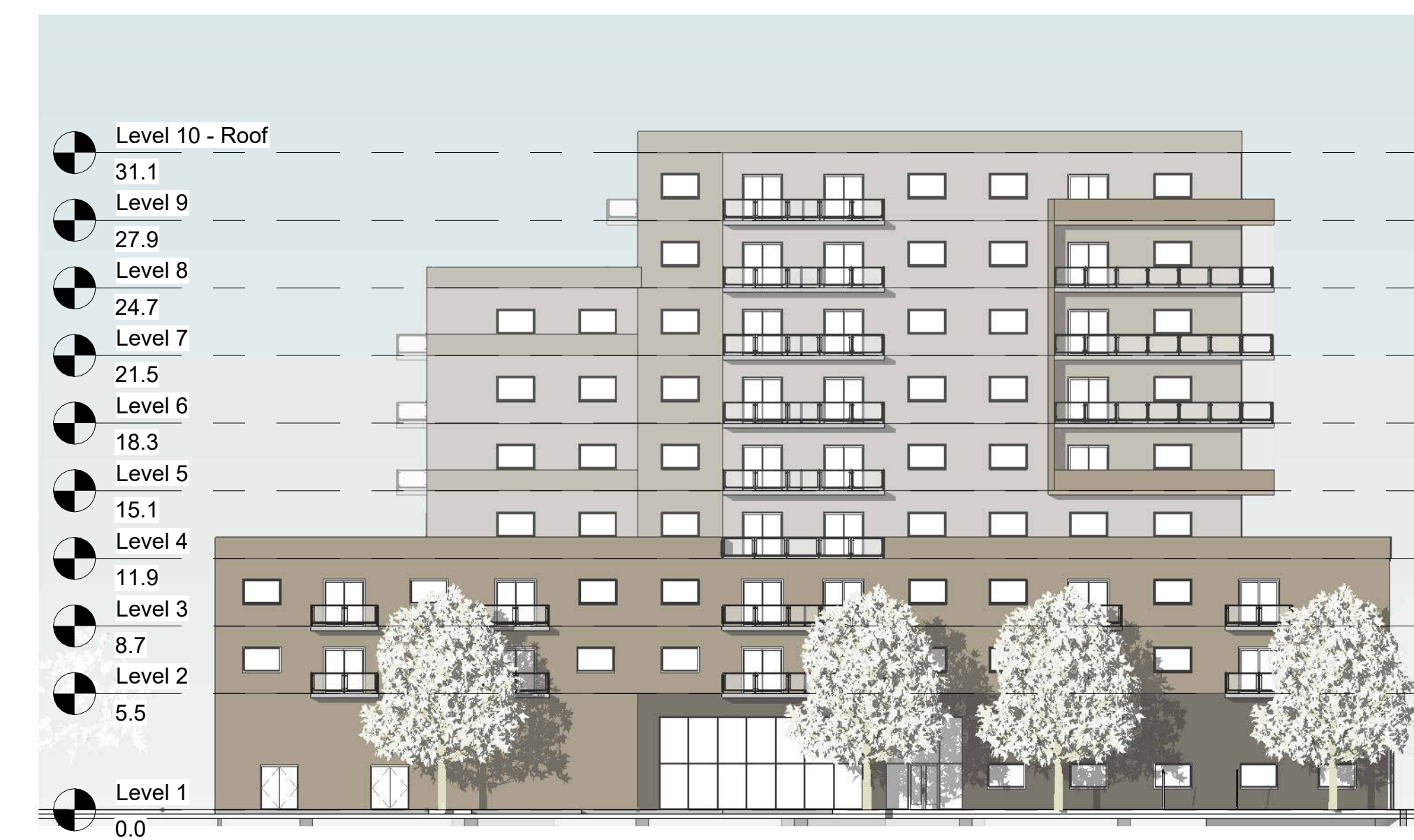
BUILDING A - EAST ELEVATION 1 : 250
