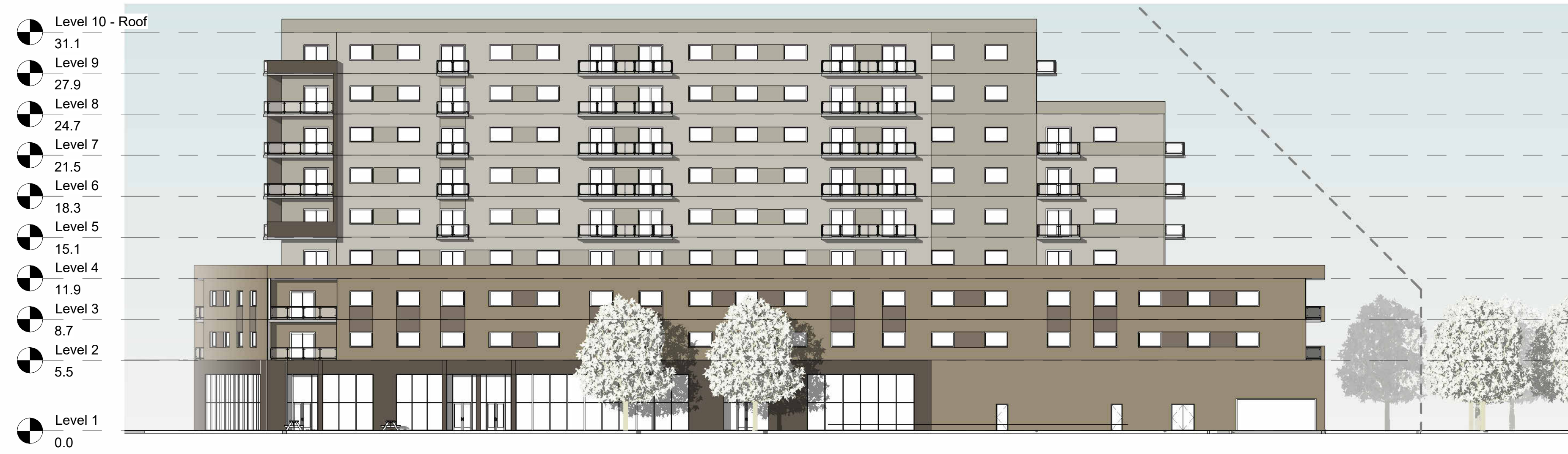
BUILDING C - WEST ELEVATION 1 : 250
