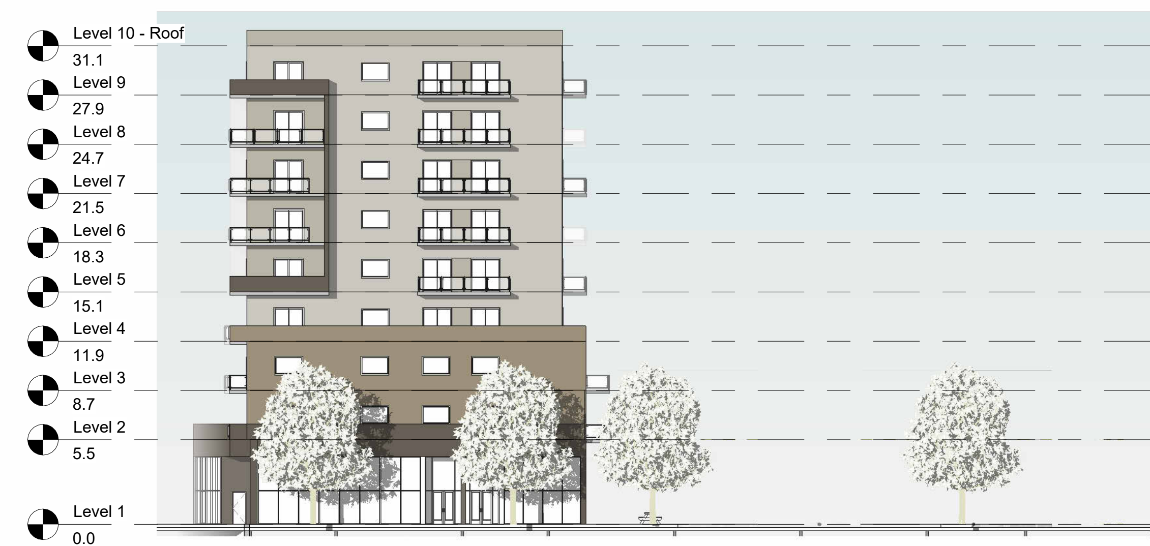
BUILDING B - WEST ELEVATION 1 : 250
