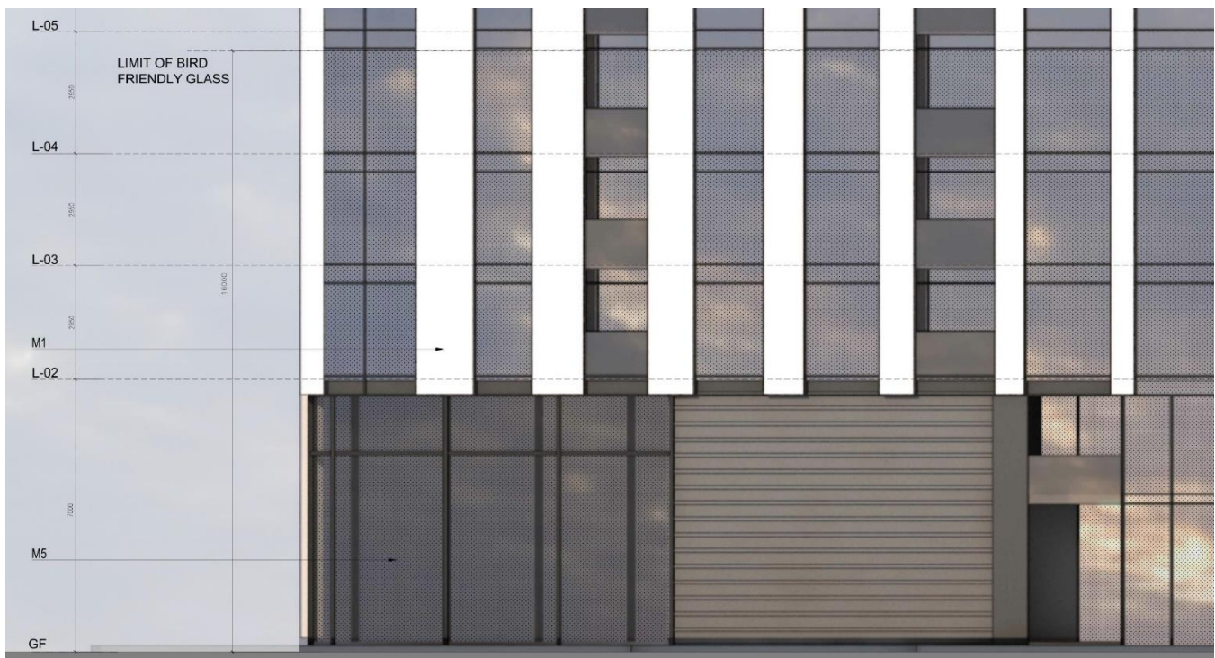
Figure 14: Bird Friendly glazing at the podium of the proposed development
