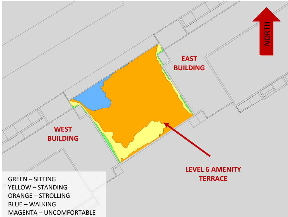
FIGURE 4A: SPRING – WIND CONDITIONS, COMMON AMENITY TERRACE
