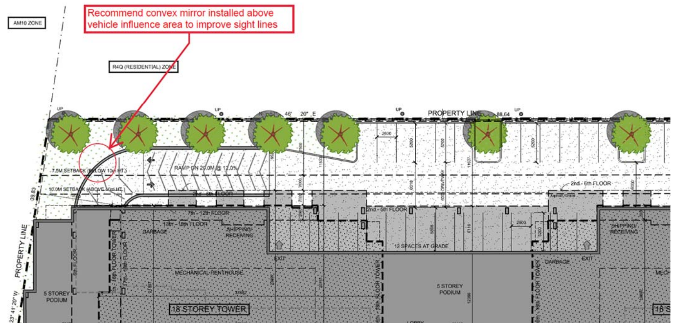
Figure 15: Parking Garage Access
