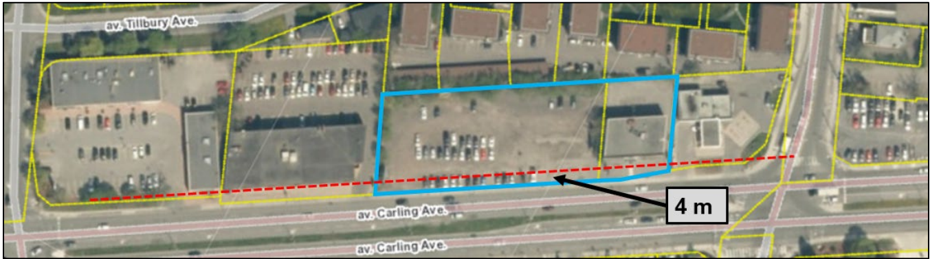
Figure 4. Reduced right-of-way dedication at 4 metres.
