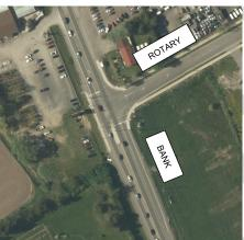
• Bank Street & Rotary Way is a 3-legged signalized intersection with auxiliary left-turn lanes on the southbound and westbound approaches, and an auxiliary right-turn lane on the northbound approach. The intersection is located immediately adjacent to the subject site and will be most impacted by the addition of site-generated traffic. The intersection will ultimately be reconfigured as a 4-legged intersection with the planned extension of Barrett Farm Drive.
