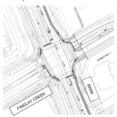
been reconstructed to accommodate the Lilythorne subdivision via a new road on the east approach which was opened to the public as a signalized intersection in fall 2019. The intersection has auxiliary left-turn lanes on all approaches and an auxiliary right-turn lane on the southbound approach. The intersection is located 730m south of the proposed development.
