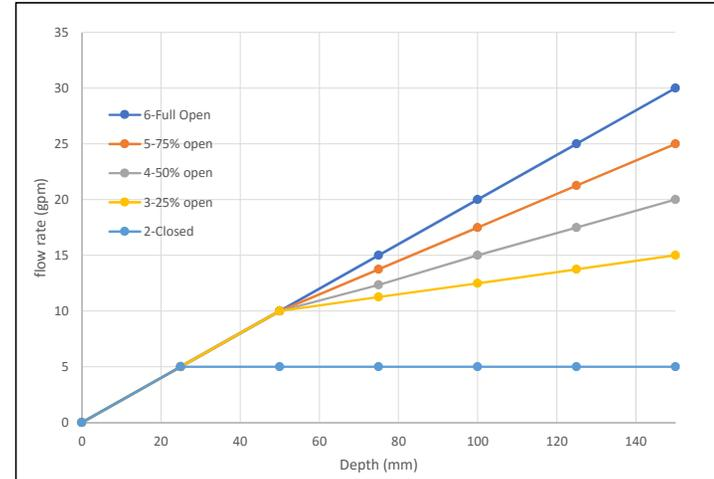
**WATTS ADJ ACCUTROL WEIR FLOW RATES (Data From Manufacturer's Catalog)**
