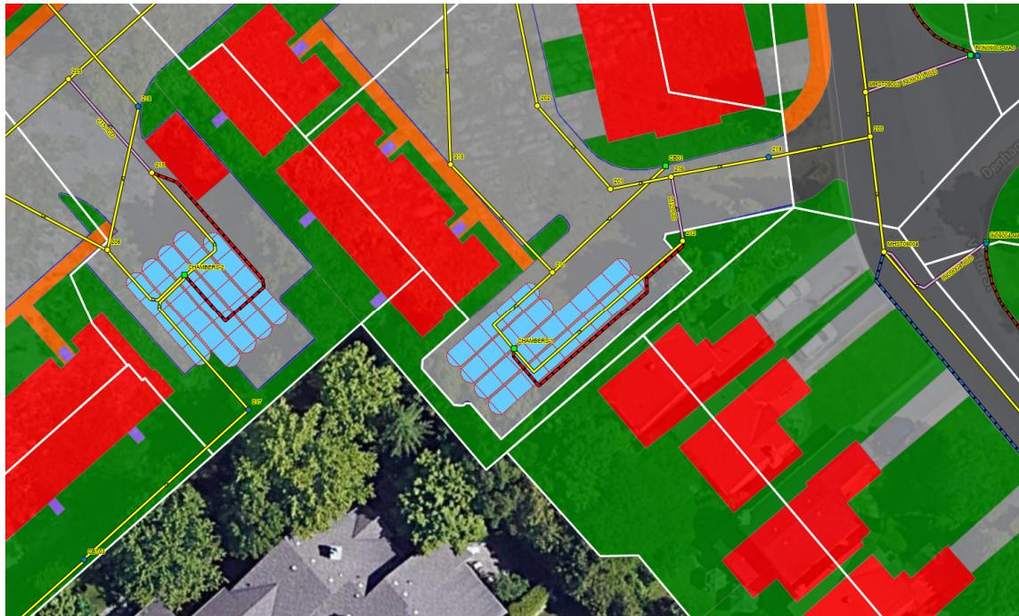
**Figure 2 - Model Schematic Illustrating Subcatchments, Links, Nodes, Outlets (ICDs)**
