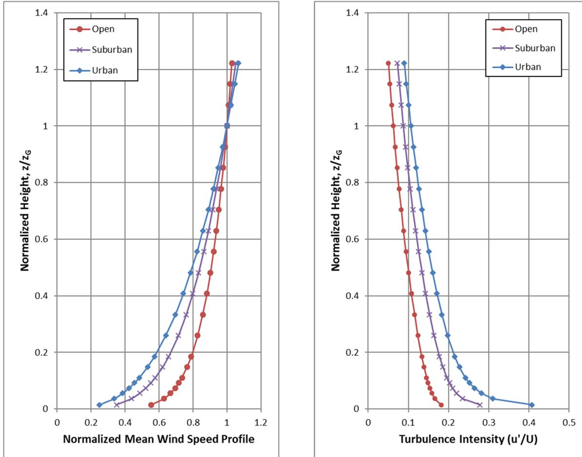
**FIGURE A1 (LEFT): MEAN WIND SPEED PROFILES;
