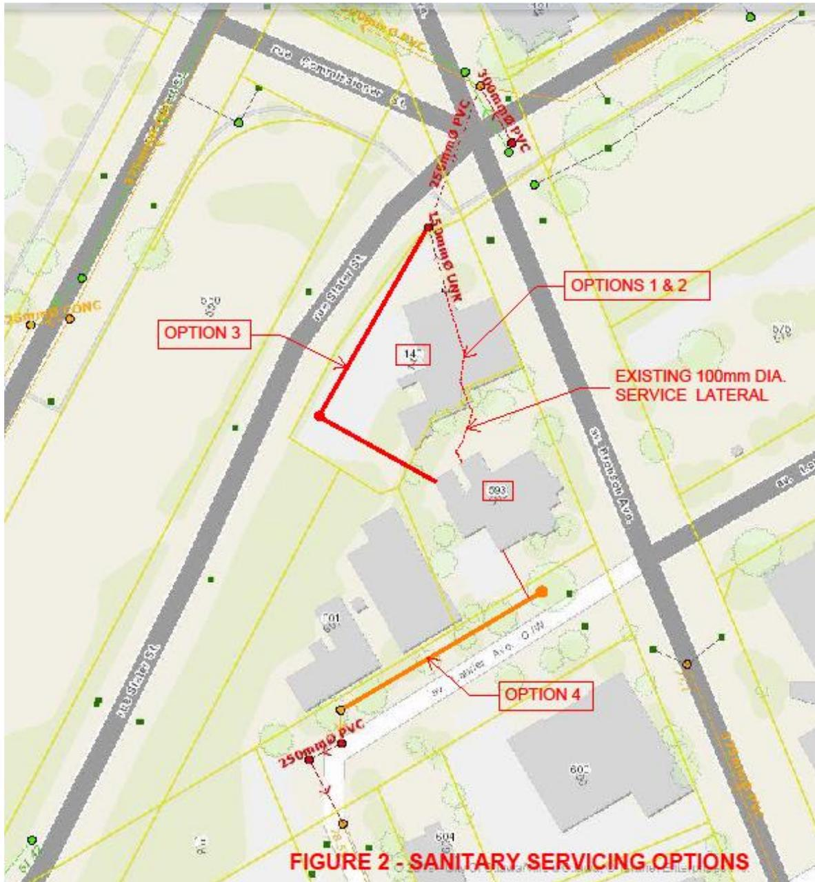
The Option 3 was chosen through discussions with the City of Ottawa. Therefore, the proposed residential development will be serviced by a new 200mm dia. sanitary sewer that will be routed through the 140 Bronson property and connected to the existing 250mm dia. sanitary sewer at the corner of Slater Street and Bronson Avenue.
