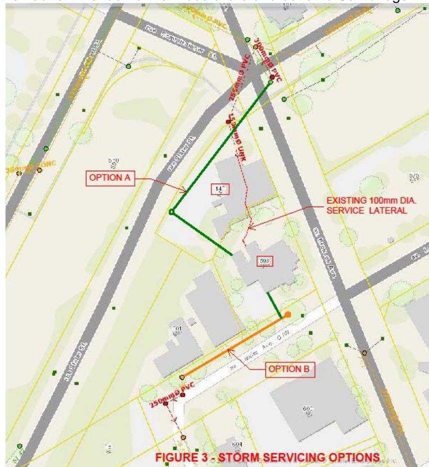
Through discussions with the City of Ottawa, a modified Option A was chosen with the outlet to the existing 250mm dia. combined sewer at the south-west corner of the intersection of Slater Street and Bronson Avenue, which in turn outlets into an 1800mm dia. combined sewer in Booth Street. The proposed storm drainage and stormwater management design for the site is discussed in the following sections of the report.
