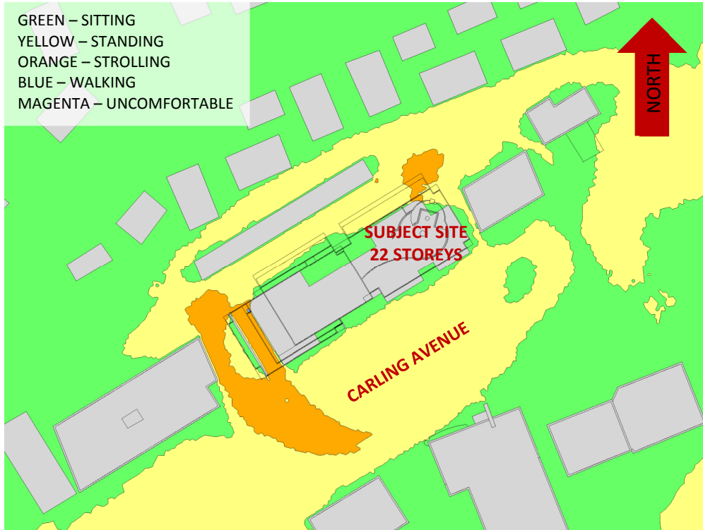
FIGURE 3A: SPRING – WIND CONDITIONS AT GRADE LEVEL
