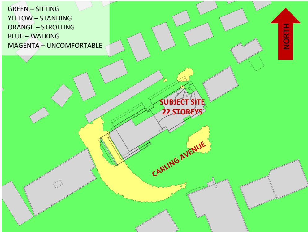
FIGURE 4A: SUMMER – WIND CONDITIONS AT GRADE LEVEL
