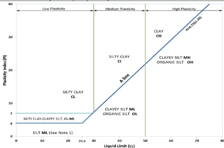
**Note 1** – Fine grained materials with PI and LL that plot in this area are named (ML) SILT with slight plasticity. Fine-grained materials which are non-plastic (i.e. a PL cannot be measured) are named SILT.
