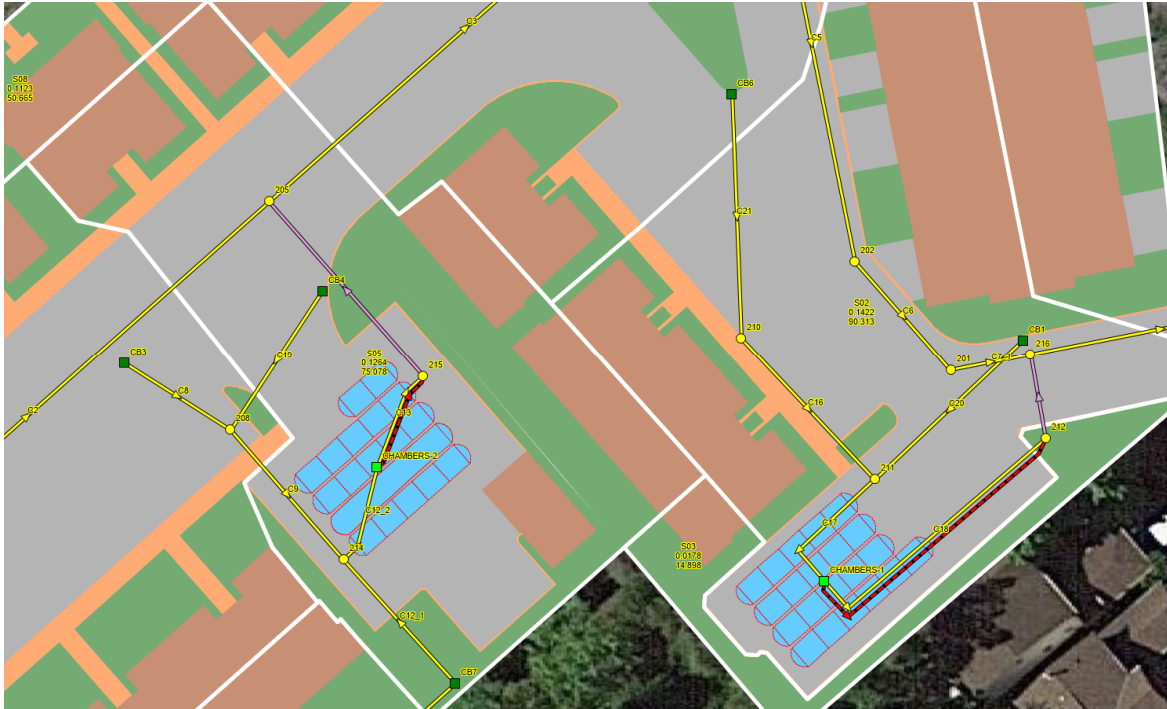
Figure 1 - Model Schematic Illustrating Subcatchments, Links, Nodes, Outlets (ICDs)
