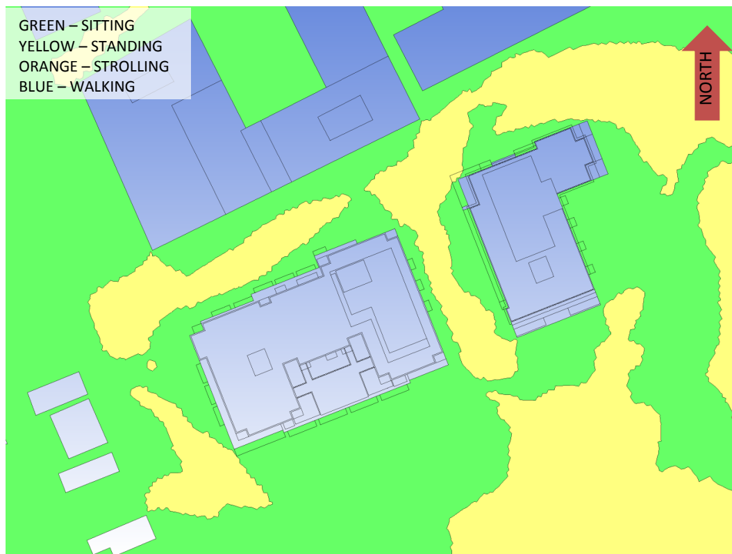
FIGURE 5A: AUTUMN – GRADE-LEVEL PEDESTRIAN WIND CONDITIONS
