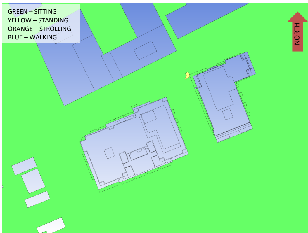
FIGURE 4A: SUMMER – GRADE-LEVEL PEDESTRIAN WIND CONDITIONS
