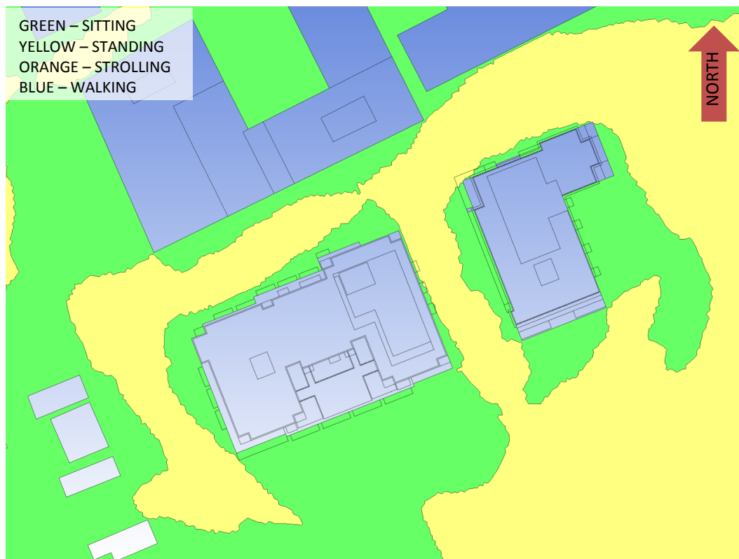
FIGURE 3A: SPRING – GRADE-LEVEL PEDESTRIAN WIND CONDITIONS
