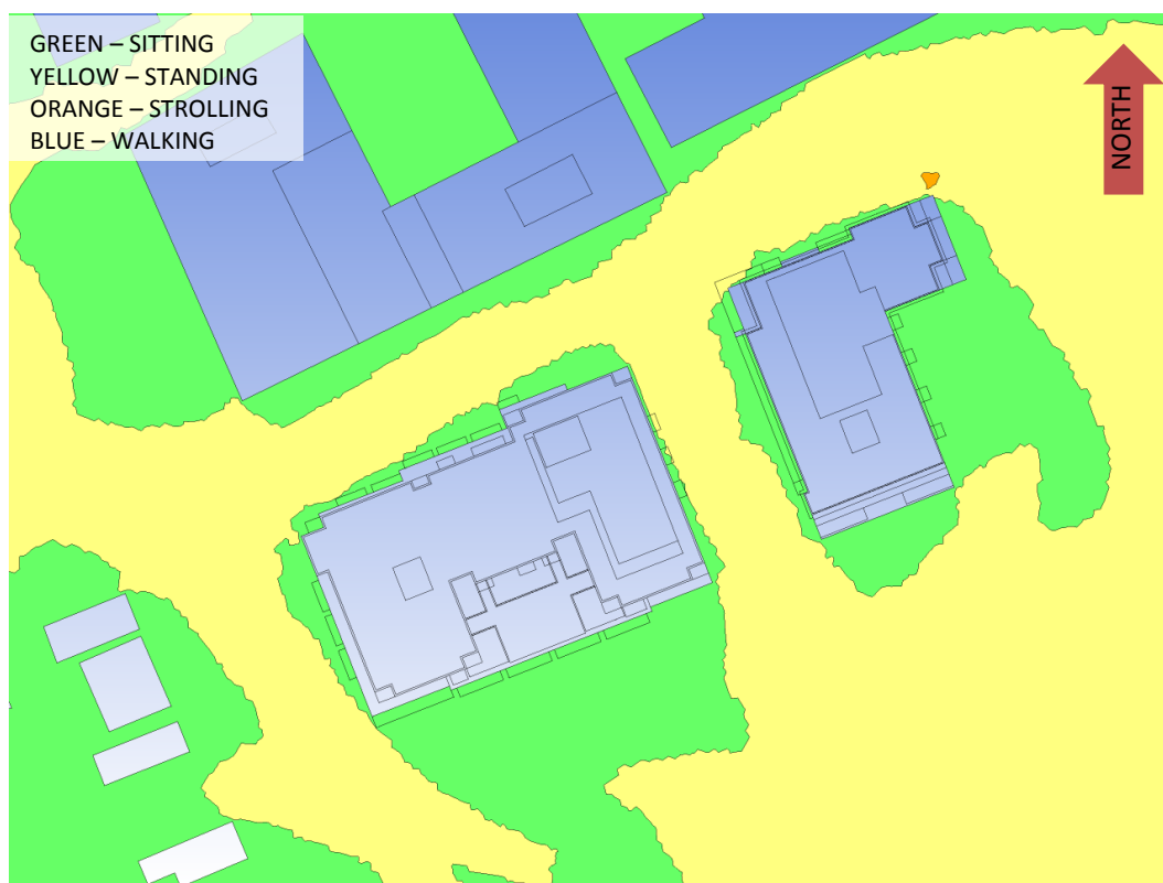
FIGURE 6A: WINTER – GRADE-LEVEL PEDESTRIAN WIND CONDITIONS
