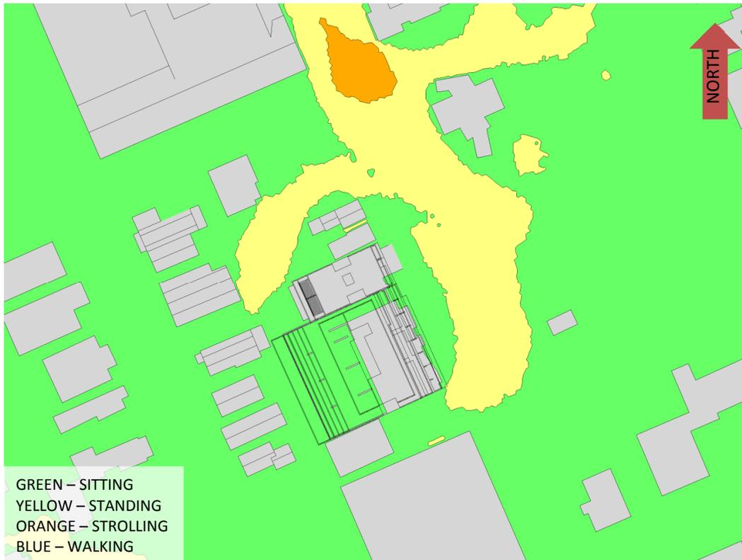
**FIGURE 3A: SPRING – GRADE-LEVEL PEDESTRIAN WIND CONDITIONS**
