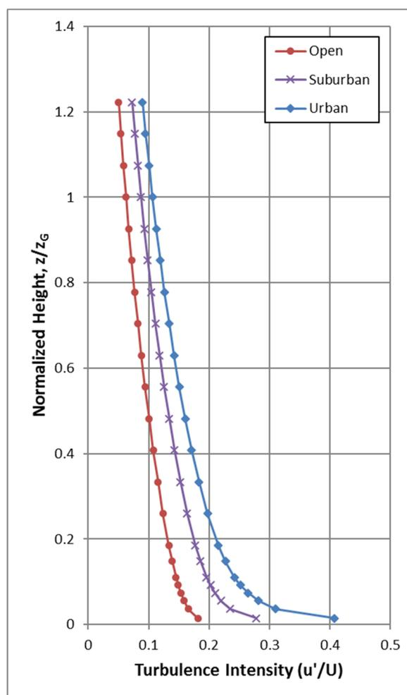
Figure A2: Turbulence Intensity Profiles
