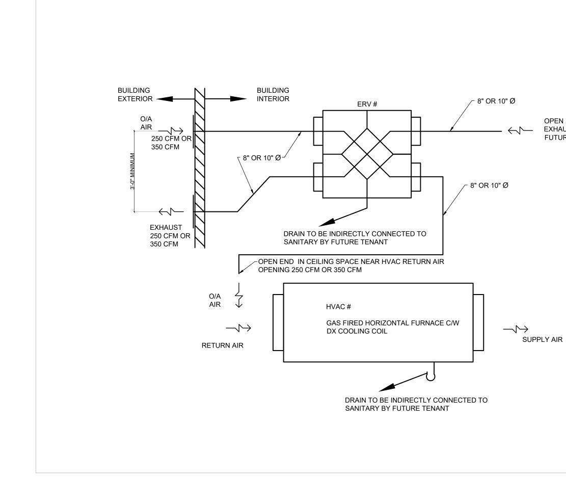
TYPICAL HVAC AND ERV DIAGRAM
