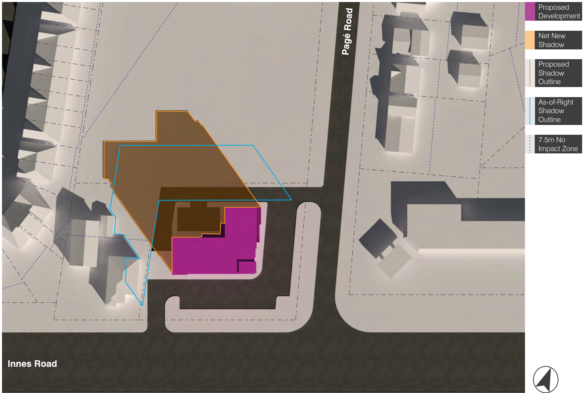
3443 INNES ROAD TOP VIEW SHADOW STUDY SEPTEMBER 21 ST 9AM EDT | 1704 | SCALE NTS | 24 OCTOBER 2017
