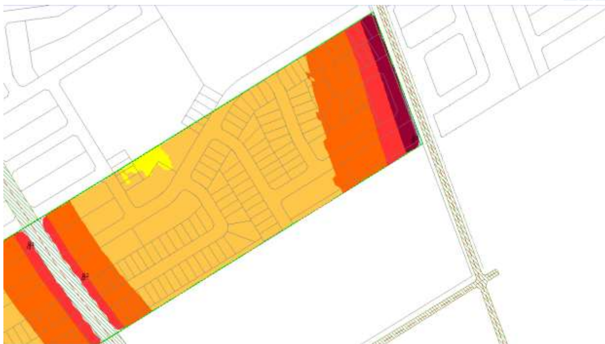
FIGURE 7: GROUND LEVEL NOISE CONTOURS FOR EASTERN HALF OF SITE (DAYTIME PERIOD)
