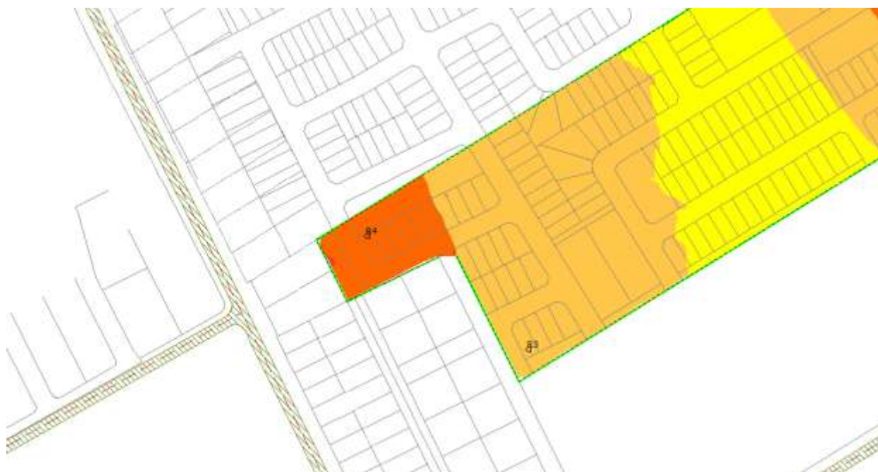
FIGURE 5: GROUND LEVEL NOISE CONTOURS FOR WESTERN HALF OF SITE (DAYTIME PERIOD)
