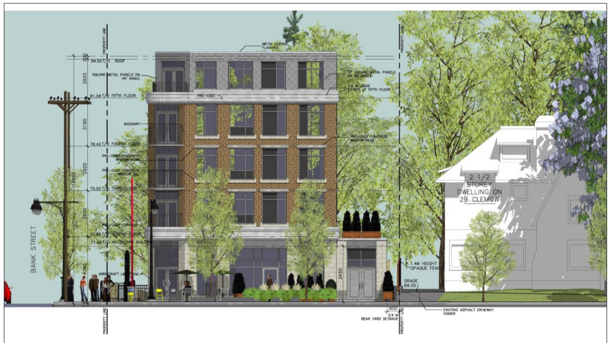
South rendering, current version, showing removal of two storeys at east side and new attached accessory building
