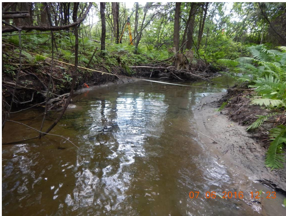
Reach 3 – downstream facing at surveyed cross-section 5 (mid-reach) – pool feature; bed material clay to sand with embedded cobbles; sand on inner bank, undercut outer bank
