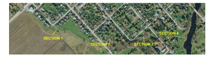
Section 1 is found in Reach 3 upstream of the VG-R3 inlet and just upstream of the Queen Charlotte Street drain. This section was selected as it represented both an erosional component (the banks are eroding and the channel is widening) and a depositional component (there is a silt accumulation on the bed). The cross-sectional plot showing the shape of the section is shown below; water elevation at the time of the survey is also indicated.
