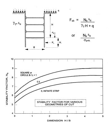
Figure 1 - Stability Factor for Various Geometries of Cut
