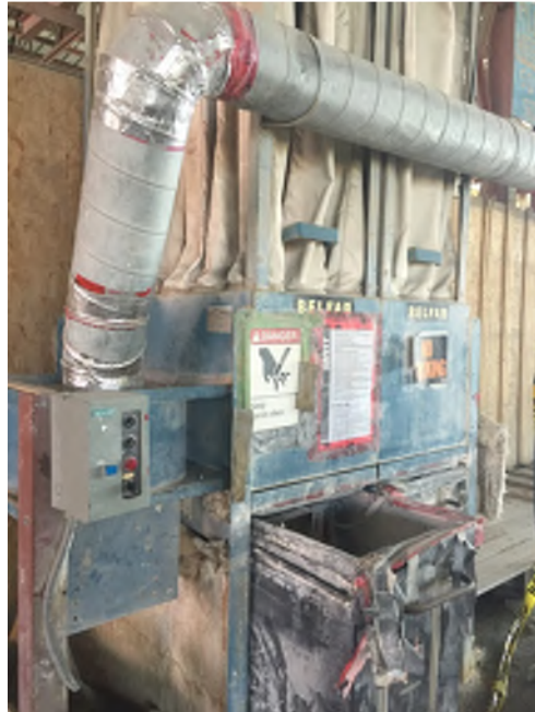
Photo 38. Saw dust collector system located in building #6.
